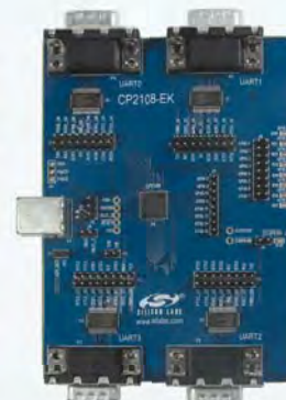
CP2108 USB TO QUAD UART EVALUATION BOARD
