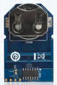
Si4010 EZRadio® KEY FOB TRANSMITTER
