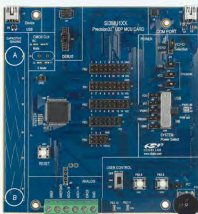
SiM3U1xx PRECISION32™ UNIFIED DEVELOPMENT PLATFORM MCU CARD
